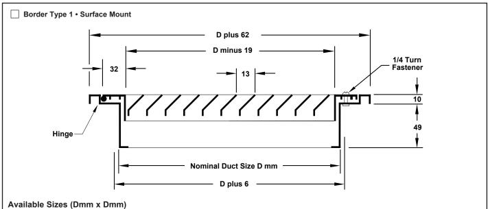
Sizes 152 x 102 through 914 x 610 in 25 increments. Border Type 3 is available in module sizes 610 x 305, 610 x 610, 914 x 305, 914 x 610 and 1219 x 610. Note: Dimensions are in millimeters.
