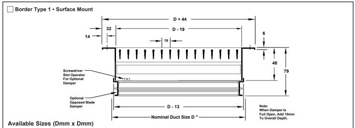
152mm x 102mm through 1219mm x 1219mm in 51mm increments in one piece construction. Odd sizes are available at additional cost. Sizes larger than 1219mm x 1219mm are shipped in multiple sections with joining strips for field assembly.
