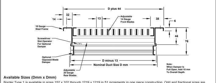
Border Type 1 is available in sizes 152 x 102 through 1219 x 1219 in 51 increments in one piece construction. Odd and fractional sizes are available at additional cost. Sizes larger than 1219 x 1219 are shipped in multiple sections with joining strips for field assembly.
