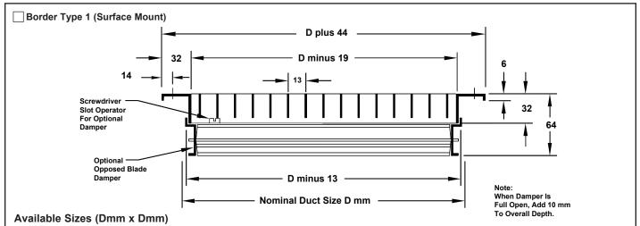
Border Type 1 is available in sizes 152 x 102 through 1219 x 1219 in 51 increments in one piece construction. Odd and fractional sizes are available at additional cost. Sizes larger than 1219 x 1219 are shipped in multiple sections with joining strips for field assembly.
