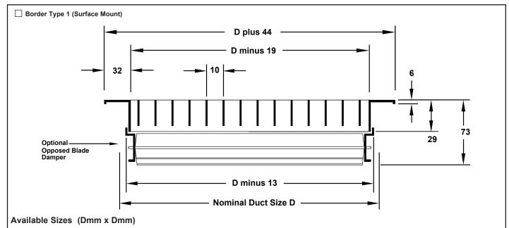
152 X 102 through 1219 X 1219 in one piece construction. Sizes larger than 1219 X 1219 are shipped in multiple sections with joining strips for field assembly. Odd and fractional sizes are available. Dimensions are in millimeters. Wall or duct opening should be duct sizes ± 3.
