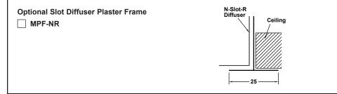
The MPF-NR diffuser mounting frame can be used in sheetrock or plaster ceiling. The frame is mounted in the ceiling by others. The Model MN-1-DR/N-4-DR diffuser is mounted on the inside lip of the frame. Plaster frame is 38 mm high.
