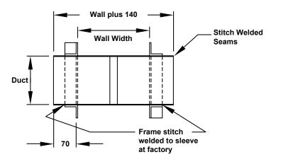
Note: Available in sizes 152 x 152 mm through 2032 x 2032 mm in one piece construction with up to a 305 mm sleeve or 1524 x 1524 mm with larger sleeve lengths. Larger sizes will be shipped in multiple sections for field welding together. Standard sleeve length = 305 mm.
