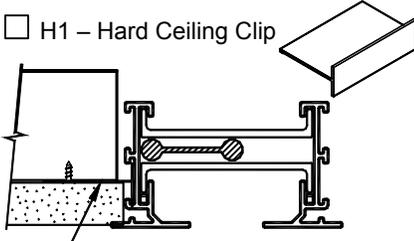
Used for mounting border type 66 with standard 5/8" gyp board.
