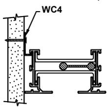
Used for flush mounting border types 66 to a wall.
