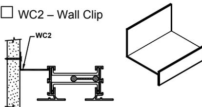
Mounts border type 66 away from a wall when a reveal is required. This reveal can be used as a return air slot.
