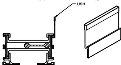
Suspends one side of the FlowBar assembly from the ceiling structure.
