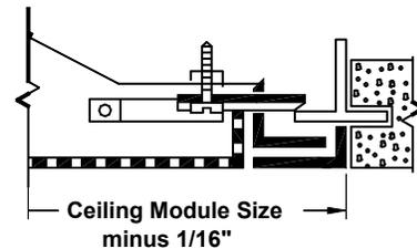
**Note:** 4SL can be installed after ceiling tiles are in place.
