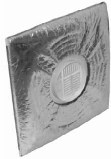
Insulation is R-6 where blanket has the most depth. One-inch clearance on each side of neck is left for insulated duct connection. 24 x 24-inch module size only. Blanket is factory installed.
