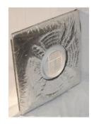
Insulation is R-6 where blanket has the most depth. One-inch clearance on each side of neck is left for insulated duct connection. 24 x 24-inch module size only. Blanket is factory installed.
