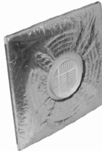
Insulation is R-6 where blanket has the most depth. One-inch clearance on each side of neck is left for insulated duct connection. 24 x 24-inch module size only. Blanket is factory installed.
