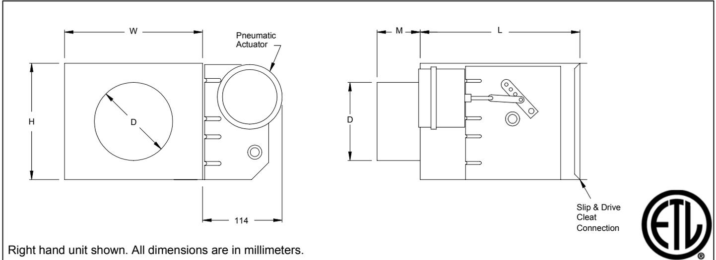
Right hand unit shown. All dimensions are in millimeters.
