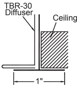
The PF-TBD slot diffuser mounting frame can be used in sheetrock or plaster ceiling. The frame is mounted in the ceiling by others. The TBR-30 is mounted on the inside lip of the frame. Plaster frame is 1 1/2" high.
