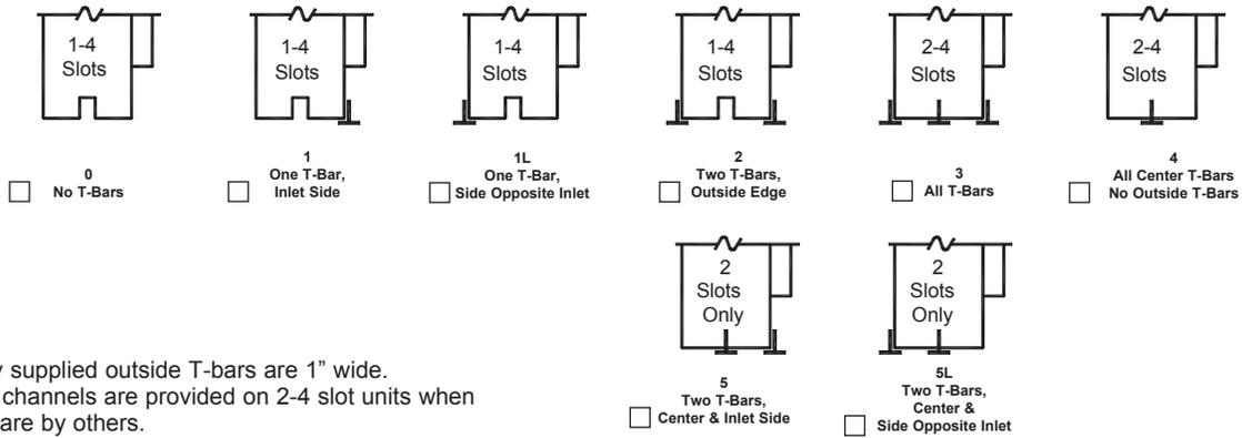
Note: Factory supplied outside T-bars are 1" wide. Center channels are provided on 2-4 slot units when T-bars are by others.
