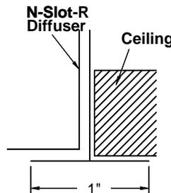
The PF-NR diffuser mounting frame can be used in sheetrock or plaster ceiling. The Frame is mounted in the ceiling by others. The model N-1-R or N-4-R diffuser is mounted on the inside lip of the frame. Plaster frame is 1 1/2" in height.
