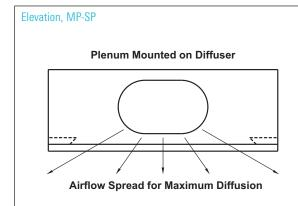
MP-SP models maximize air diffusion by shortening the throw and widening the spread of the discharge air. This is accomplished by internal baffling. The result is improved comfort in short-throw applications, as in exterior zones.
