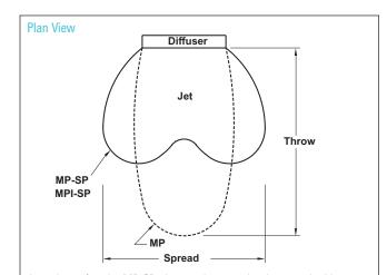
At a given cfm, the MP-SP plenum shortens the throw and widens the spread of the air leaving the diffuser (as compared with the MP plenum or standard plenum).
