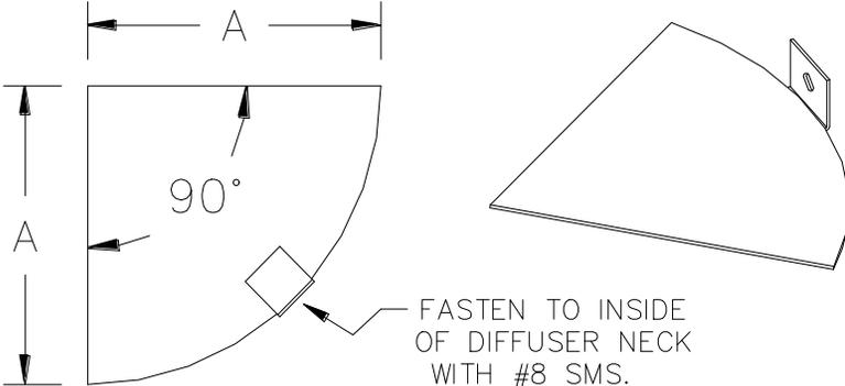
FASTEN TO INSIDE OF DIFFUSER NECK WITH #8 SMS.
