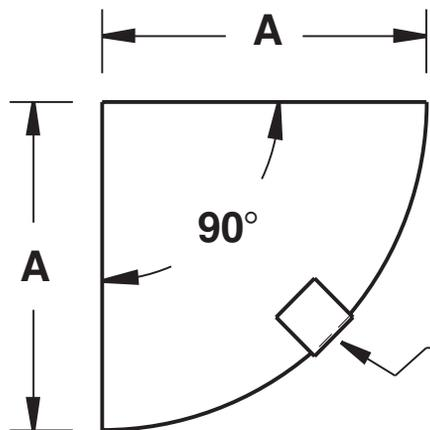
**Fasten to inside of diffuser neck with #8 SMS. (by others)**
