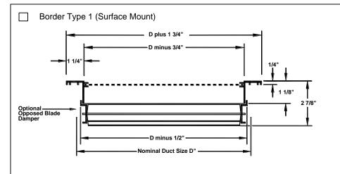
Border Type 1 available in sizes 6" x 4" through 48" x 48" in one piece construction. Sizes larger than 48" x 48" are shipped in multiple sections with joining strips for field assembly. Odd and fractional sizes are available at additional cost.
