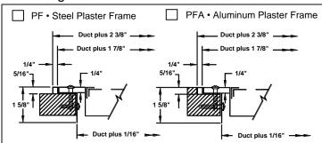
Surface Mounted Example Recessed Mounted Example Note: Wall opening should be listed duct size + 1/8". Plaster frame can be installed as either surface mount or recessed.
