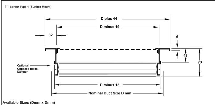
$152 \times 102$  through  $1219 \times 1219$  in one piece construction. Sizes larger than  $1219 \times 1219$  are shipped in multiple sections with aluminum joining strips for field assembly. Odd and fractional sizes are available. Wall or duct opening should be duct size  $\pm 3$ .
