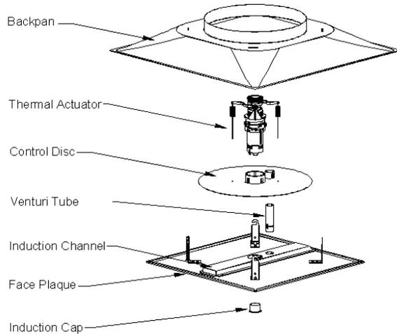
The thermal T<sub>3</sub>SQ uses a center mounted induction cap to accurately measure the room temperature. This eliminates the need for a wall mounted thermostat or sensor and provides the fastest, most accurate way of measuring the room air temperature.
