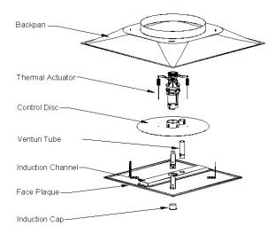
The thermal  $T_3SQ$  uses a center mounted induction cap to accurately measure the room temperature. This eliminates the need for a wall mounted thermostat or sensor and provides the fastest, most accurate way of measuring the room air temperature.
