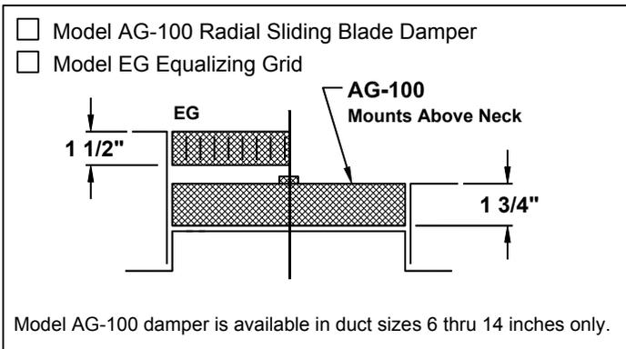
Model AG-100 damper is available in duct sizes 6 thru 14 inches only.
