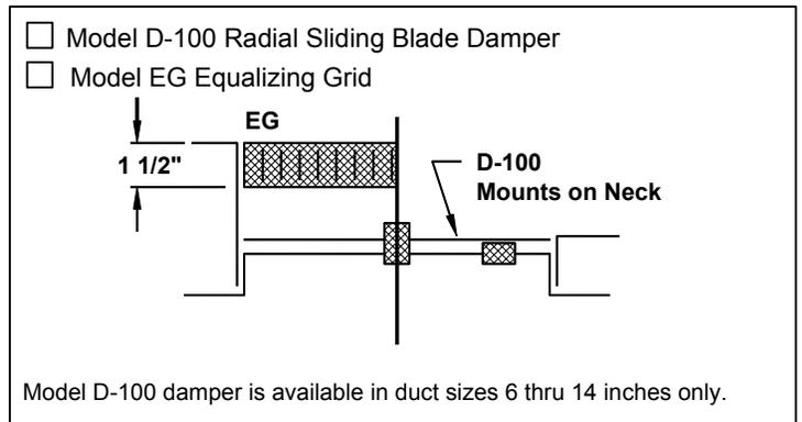
Model D-100 damper is available in duct sizes 6 thru 14 inches only.
