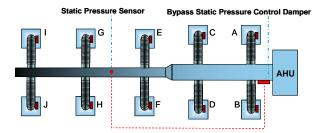
Balancing the  $T_3SQ$  VAV system is simple. First, drive open all diffusers. For the thermal  $T_3SQ$  this is done by disconnection the actuator arms from the control disc. For the analog  $T_3SQ$ , press and hold the down arrow to put the diffuser in override mode, signified by a "LI" on the thermostat display, then press the down arrow once to drive the control disc open.
