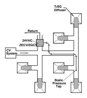
In discharge pressure control applications, the static pressure tap should be placed downstream of the terminal about  $^{1}/_{2}$  to  $^{2}/_{3}$  the way down the duct run.
