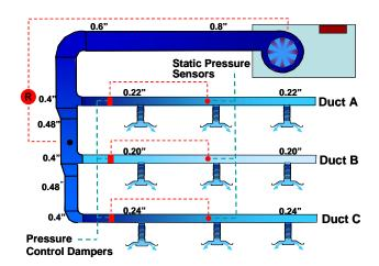
Begin by selecting the index duct. This is the duct requiring the highest static pressure. In the figure above, the index duct would be branch duct "C".
