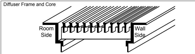
CT-TAF-L is only available with Type 5 Heavy Duty CT Floor Frame. Diffuser core is a combination of CT-PP-0, CT-481, and CT-PP-3 Core (0°, 15°, and 30° Deflection).
