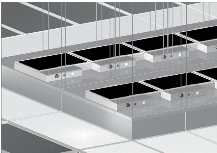
NOTES: Shown left is a typical installation of multiple fan filter units mounted above the service area, completely blanketing the critical area with clean, filtered supply air. For spot applications, a single fan filter unit can be mounted over a work bench or table to reduce particulate counts.
