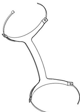
Nylon cable ties to secure flex duct to FlexRight (ties by others)
