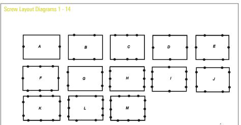
Note 1: This chart provides general information concerning location of screw holes. Screw hole location is subject to change without notice. Titus does not recommend pre-drilling mounting surfaces for screws. Use the grille as a template. This chart applies to border type 1 only.
